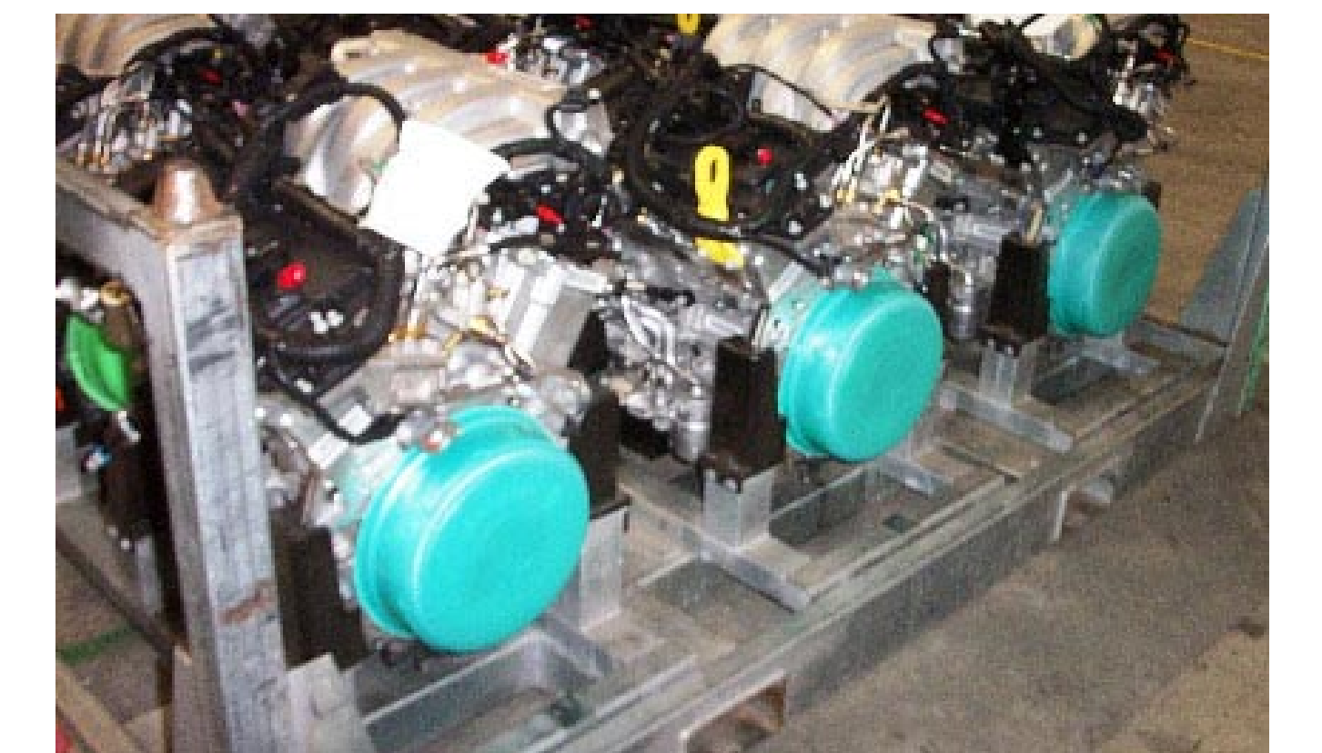
VCI corrosion inhibitors in mono and co-extruded rigid plastic protecting clutch / flywheel
