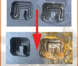
This cast steel test subject was lightly coated with G16 on the left before being fully exposed to the elements. THe bottom image shows results after 1500 hours (65 days)
